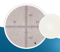
■ Membrane A: Class 4: no oxidation, no sludge. Membrane B: Class 12: a lot of sludge.
