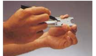
Apply mark in window using insertion gage.
