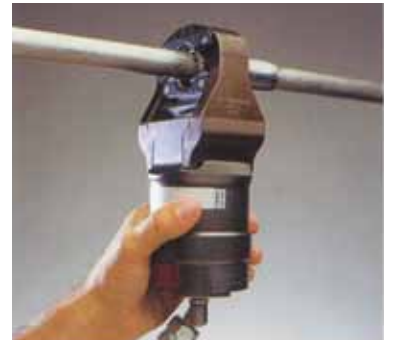
Position PYPLOK® tooling around fitting assembly and pressurize.
